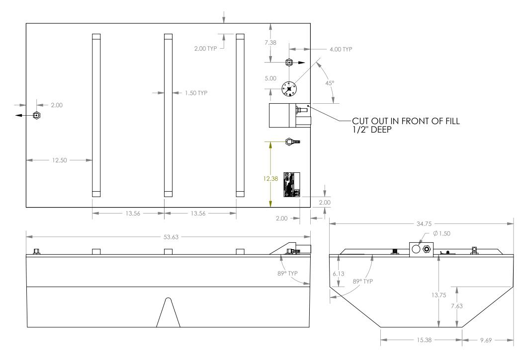
NOTE: DOGHOUSE IS 5.0 LONG, 4.50 WIDE, AND 2.50 TALL W/ A 1.25 TOP FLAT RIBS ARE 1.0 TALL, 1.50 WIDE, 2.00 FROM TANK EDGES AND BEVELED 45° AT EACH END. BAFFLES ARE 4.50 TALL. ALL DIMESIONS ARE TYPICAL FILL IS Ø1.50 X 2.75
