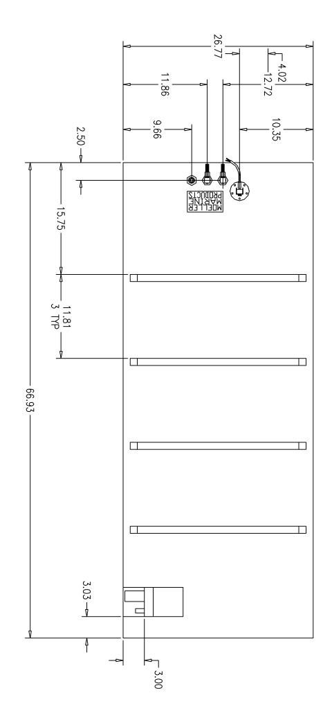
NOTE: DOGHOUSE IS 4.13 WIDE, 5.45 LONG, 2.00 TALL AND HAS A TOP FLAT OF 1.25. RECESS IN FRONT OF DOGHOUSE IS 0.50 DEEP. RIBS ARE 1.00 WIDE, 1.00 TALL, 1.00 FROM EDGE, AND ARE BEVELED 45° AT ENDS.
