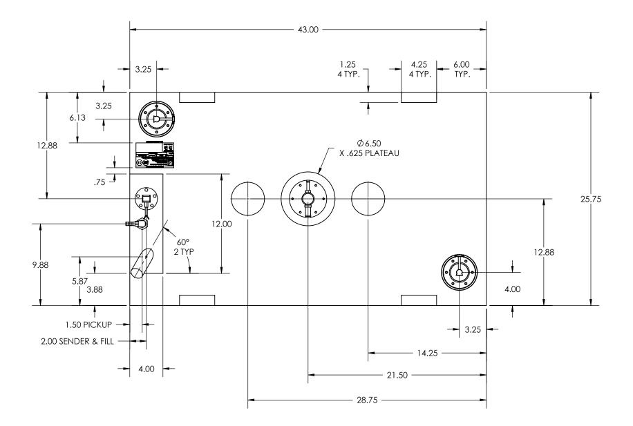
NOTE: CONES ARE Ø4.00 AT TOP OF TANK Ø5.00 AT BOTTOM OF TANK.
